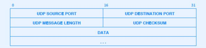
• If *UDP CHECKSUM* field contains zeroes, receiver does not verify the checksum
